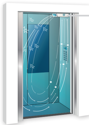
Example of installation of the JONIX up in device on lift.
