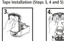
Clean installation surface with an alcohol pad. Allow surface to dry for 60 seconds. Peel paper off installation tape.
